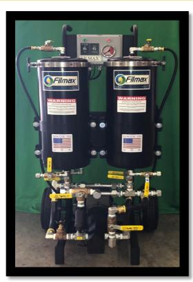
The Filmax FP2108P High Performance Portable Filtration System is proven to reduce operating and maintenance costs at 360 filtered gallons per hour
